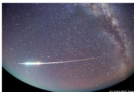
Fig. 5: Reentry fireball of the Hayabusa spacecraft and the capsule. This photographic observation was carried out using Nikon D40x with a fisheye lens (f=10.5mm/F2.8) with the exposure time of 3 minutes.
