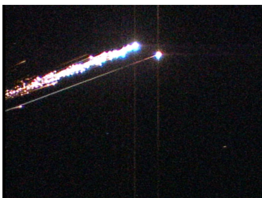
Fig. 7(b): A single frame image (1/30 s) of the reentry capsule (the right front) and fragmented Hayabusa spacecraft are captured by NC-R550a, EMCCD color TC.
